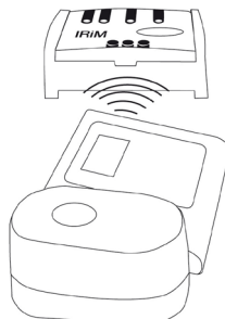
notch for IR data transfer
