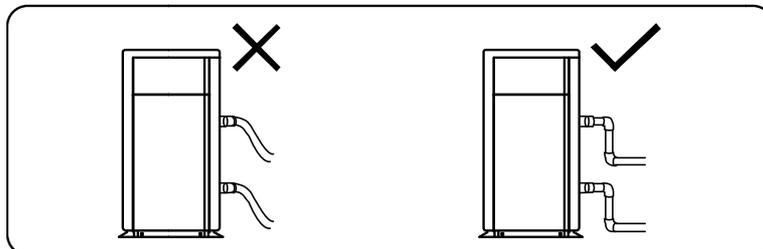
2.1.2. In order to guarantee the heating efficiency, the water pipe length should be  $\leq 10\text{m}$  between the pool and the heat pump.
